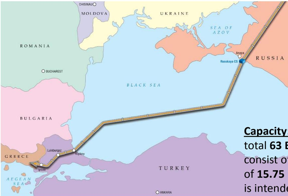
**Route:** 660 km of the offshore pipeline route will be laid within the old corridor of South Stream and 250 km – within a new corridor towards the European part of Turkey. The onshore gas pipeline section will stretch for 180 km from the Black Sea coast of Turkey to the border between Turkey and Greece.
